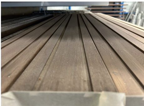
Boardwalk of Conservation Timber from Selva Maya (Pucté) in production for use in Rotterdam (Photo: Arjan De Jong, GWW Houtimport)
