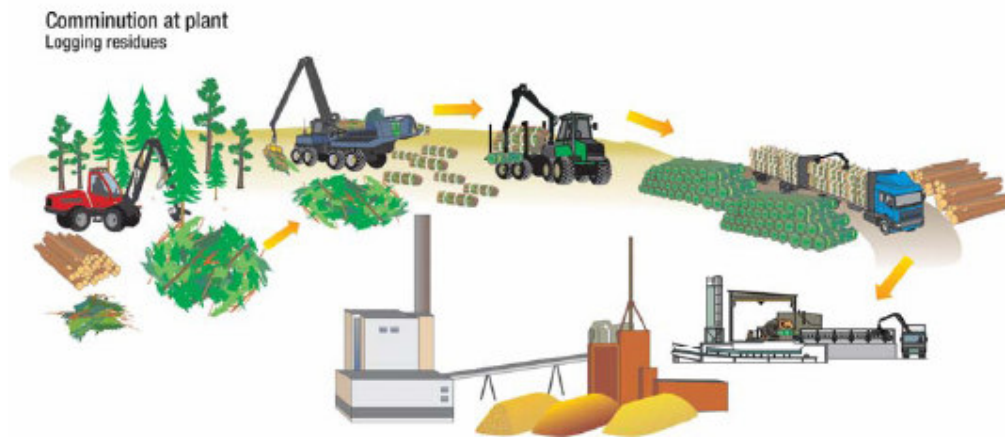
Figure 1. The bundling method the most recent developed method to extract forest residues from the forest stands (Alakangas, VTT)
