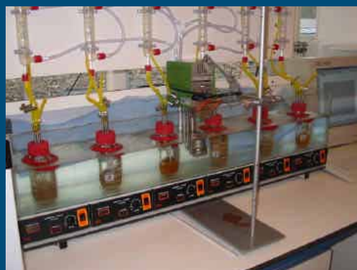
Lab-schaal ethanol fermentaties na enzym. hydrolyse
