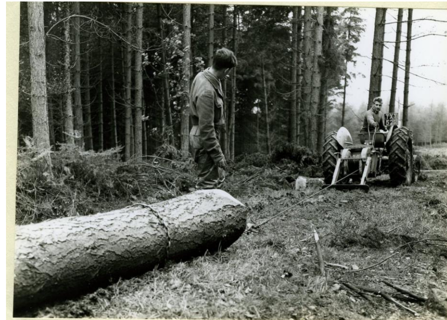
Photograph 2. The winch on the 3 point linkage of a Ferguson 35 tractor hauling timber at Alice Holt.
